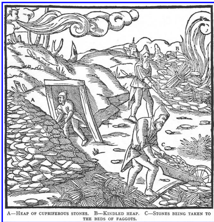
Figure 13. Method of roasting copper-bearing ore. Bundles of sticks, twigs and branches are laid out, ore is laid over them, then more layers until a mound is formed. Firing is on the right side, away from the wind (note the wind, top left) in order to prolong the burning. These piles might burn as long as thirty days (31). (Agricola, De Re Metallica, Public Domain).
