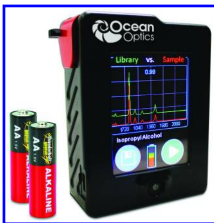
Figure 5. A Portable Raman Spectrometer Measuring 9.1 X 7.1 X 3.8 cm. Courtesy Ocean Optics.
