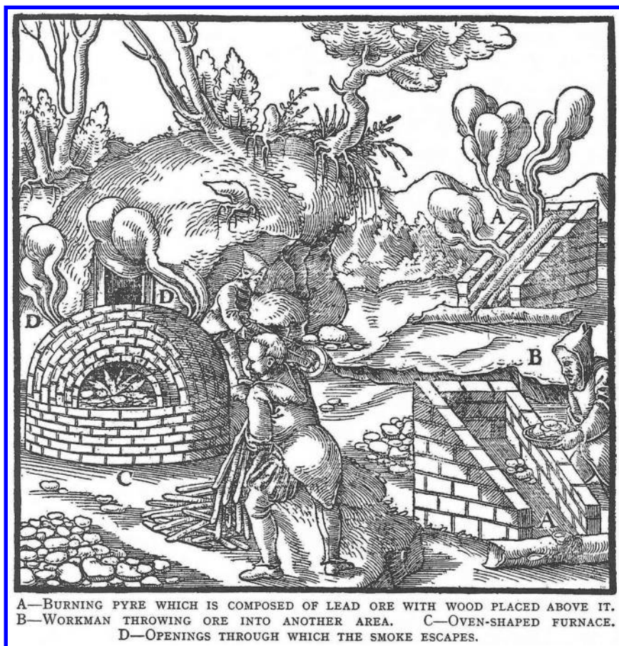
Figure 19. Roasting and smelting lead ore. The ore is roasted in a sloping furnace with logs that are placed on top of the ore. The slope allows the melting lead to flow out of the furnace. It is further refined in the covered furnace (40). (Agricola, De Re Metallica , Public Domain).
